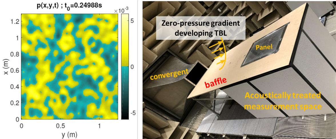
Figure 1: (Left) A realization of the wall pressure field in the case of a diffuse acoustic field excitation; (Right) The experimental setup used for measurements in wind-tunnel.
