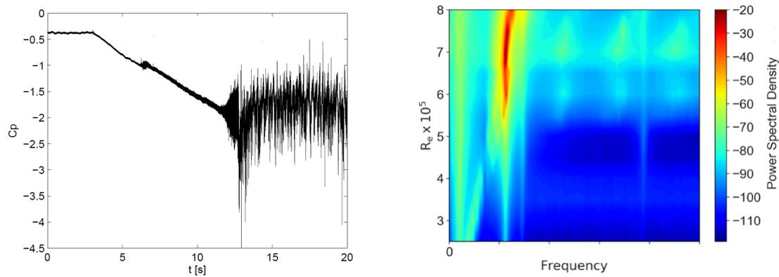
Figure 1: Left; Experimental transient time series of the wall pressure coefficient close to the leading edge on the suction side of a hydrofoil undergoing a pitching transient motion. Right; Experimental vibration level of a rectangular plate versus frequency and Reynolds number.
